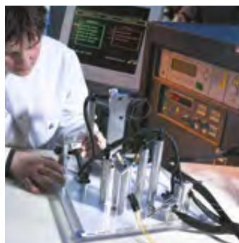
▲ AUTOMATIC CONTINUITY & INSULATION RESISTANCE TEST
