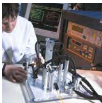
▲ AUTOMATIC CONTINUITY & INSULATION RESISTANCE TEST
