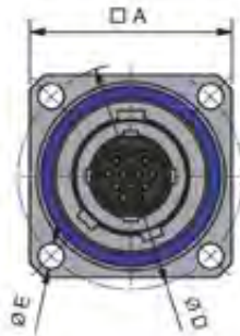
Rear mount square flange female PCB 0.050" pitch MCABKxxx-10S50Sxxx
