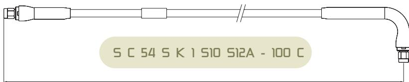
5.4 mm diameter CELLOFLON® Axowave™ made with a single-stranded Axowave™ cable insulated with FEP, terminated with a SMA plug connector and a 90° swept SMA connector, 1 m length.
