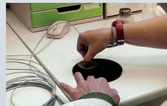
HAND POLISHING ON OPTICAL CONTACT IN THE AXON' OPTICAL LABORATORY
