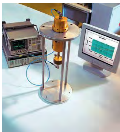
EMI PROTECTION : TRANSFER IMPEDANCE MEASUREMENT
