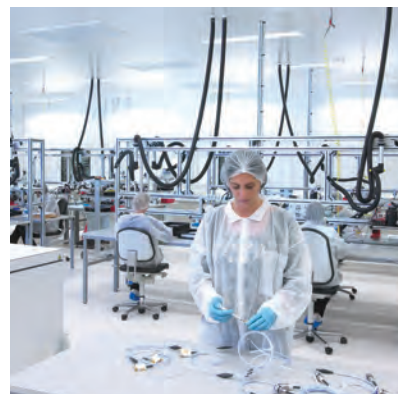
MANUFACTURE OF HARNESSSES IN ISO 8 CLEAN ROOM
