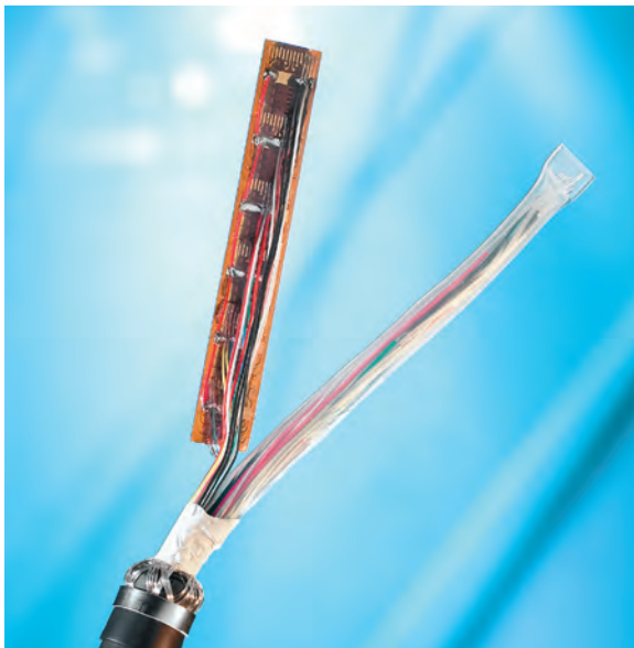
Picocoax ® wires soldered onto a PCB
