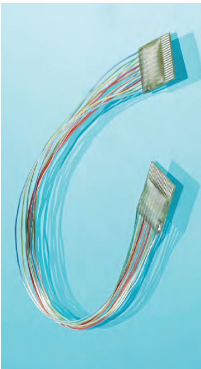
Picocoax ® wires connected to Printed Circuit Boards
